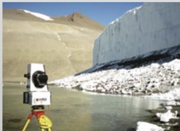
I-SiTE 4400 set up at base of glacier
