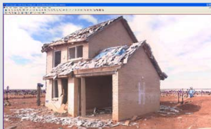
Damage to the house in terms of its overall stability, as well as the destruction of individual materials, can be clearly seen on images acquired and registered automatically to the 3D data by the I-SiTE 4400
