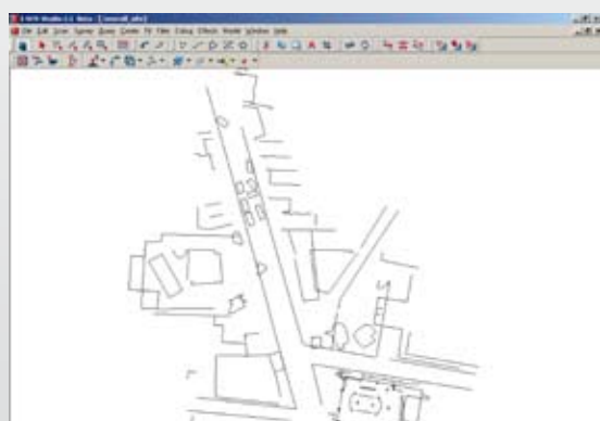
2D plan built from scan data
